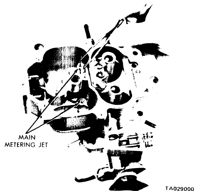
Figure 12-7. Removing or Installing the Main Metering Jets. (15) Remove the venturi cluster screws to lift the venturi cluster and gaskets up and away from the main body (figure 12-8). Discard the gaskets.
