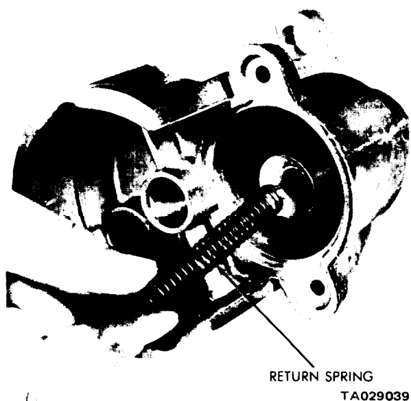
Figure 15-12. Removing Return Spring.
