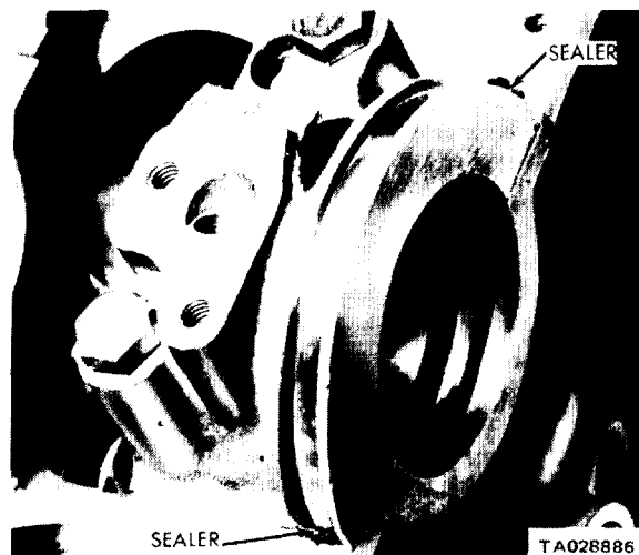
Figure 3-13. Oil Pan End Seal at Rear Bearing.
