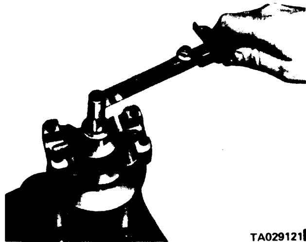
Figure 20-15. Checking Pinion Bearing Preload.
